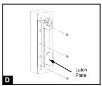
Smooth lower side seals into position, align holes in lower spring anchor brackets with holes in lower side seals (Fig. D). Secure each bracket using three 6mm x 50mm gold self tapping screw. There is no need to pilot drill for these screws.
