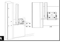
Fit pivot arms to plates in bottom corners of door using four no. 12 x <sup>3</sup>/4" self tapping screws per side Using outer holes shown. (See Figure A) 6
