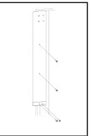
Stand door, safely propped, centrally between side jambs on two wedges. A gap of approximately 12mm (1/2") should be left between the top of the door and the lintel
